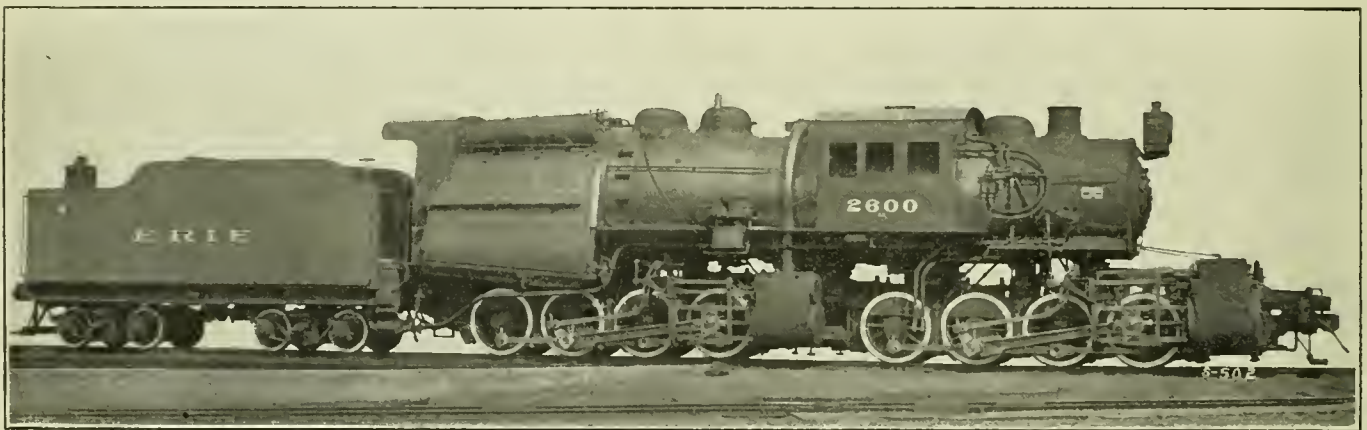
FIG. 1.—MALLETT ARTICULATED COMPOUND LOCOMOTIVE OF THE TYPE TESTED ON THE ERIE RAILROAD.
